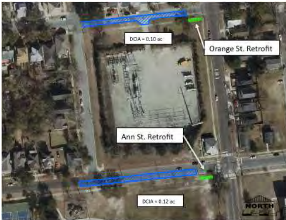
Figure 10: Orange Street and Ann Street retrofit sites with directly connected impervious areas (DCIA) in blue
