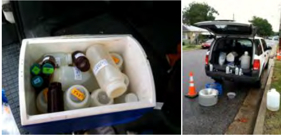
Figure 3-8: Sample bottles placed on ice for transport (left) and research vehicle with sampling equipment (right)
