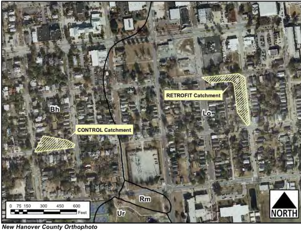
Figure 2-1: Control and LID retrofit drainage areas in Wilmington, NC
