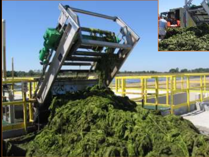
The harvested algae is removed from the water with a Flex Rake.
