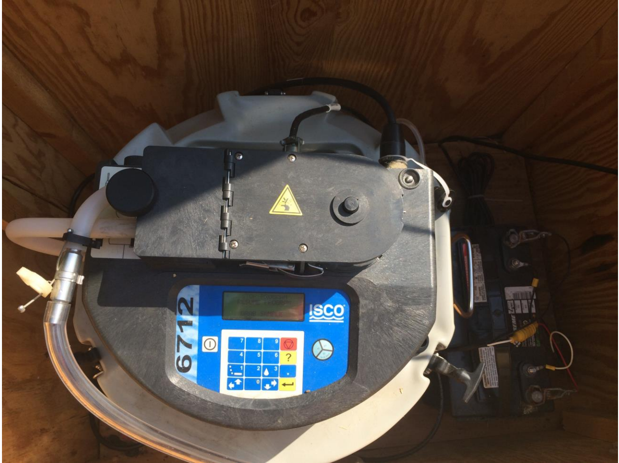
Figure 4. ISCO 6712 automatic samplers used for water quality monitoring at AAuto.
