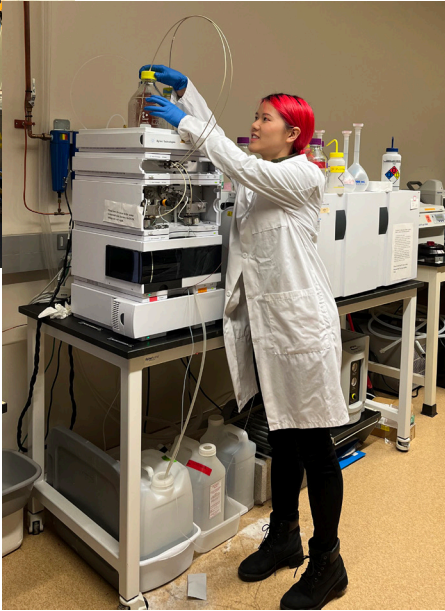
→ Mei Sun (UNC Charlotte) is utilizing an Ultraviolet-Sulfite treatment to degrade PFAS while lowering the risk of contaminating the surrounding environment. Pictured here is Postdoc Yingying You preparing the instrument for analyzing PFAS in waste samples.
